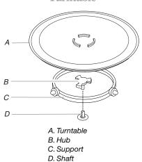
The turntable rotates in both directions to help cook food more evenly. Do not operate the microwave oven without the turntable in place. See "Assistance or Service" to reorder any of the parts.
